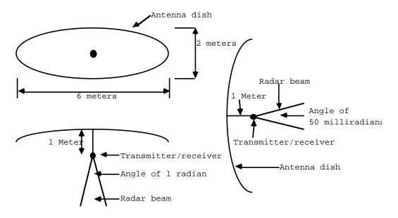
Figure 1. Measurements for the radar system.
